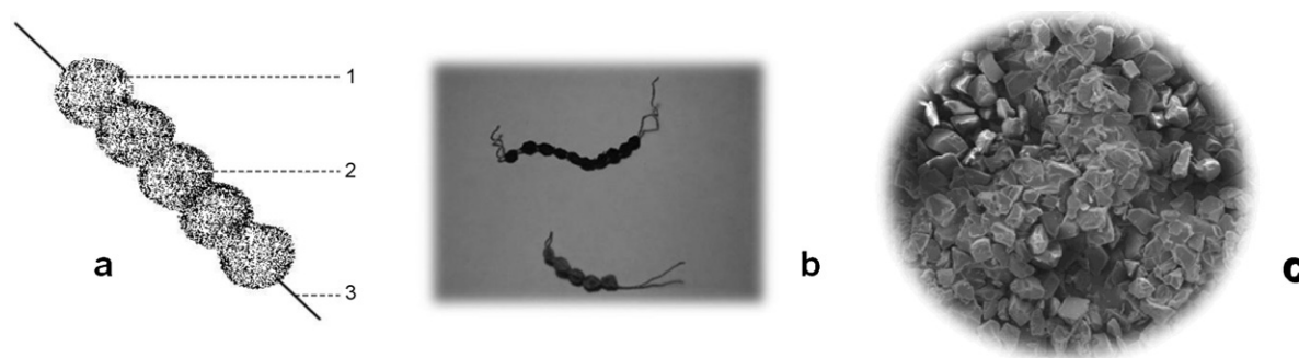
Fig. 2. Schematic representation (a), images (b) and a FE-SEM micrograph (c, 35 \times ) of the MSA \mu E device proposed in the present work [21]. 1: Polystyrene supporting spheres; 2: sorbent phase; 3: thread.
